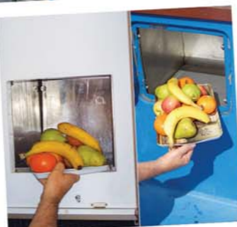
Dumb waiter with intercom transports between kitchen & top deck
